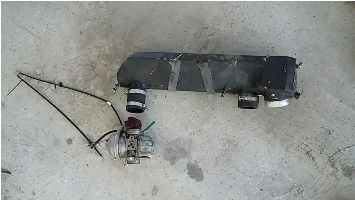
The airbox with the air filter assembly which was sucked inside
