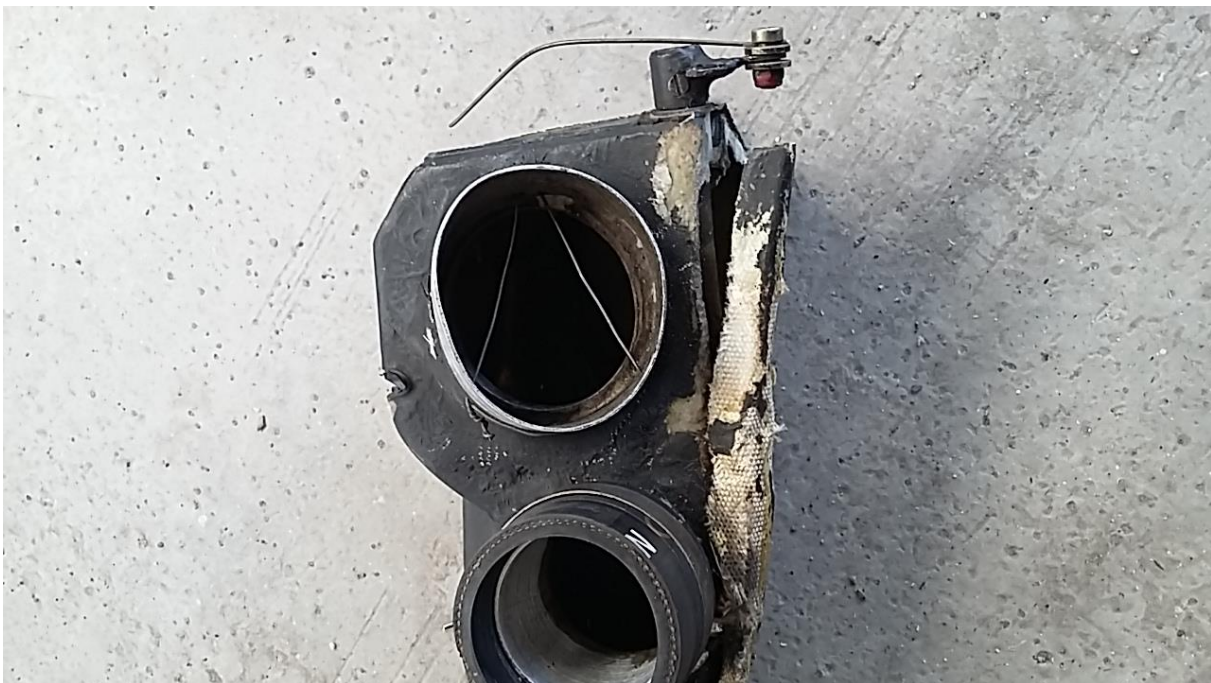
The wires which hold the air filter inside the hose during the operation
